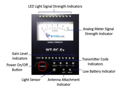
**Power On/Off Button:** Hold this button to turn on or turn off the receiver.
